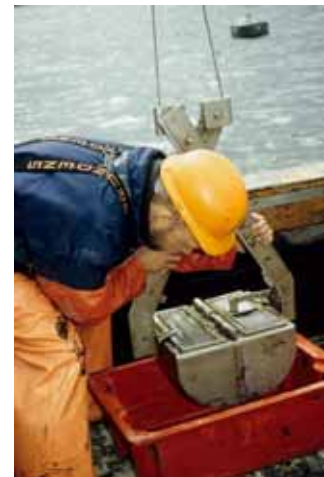
COLLECTING SEDIMENT SAMPLES WITH A VAN VEEN GRAB. SOURCE: K. BLACK/SAMS
