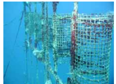
VIEW OF A HORIZONTAL ARRAY OF BIOFILTERS DEPLOYED IN THE BIOFAQS TESTS. SOURCE: K. BLACK/SAMS
